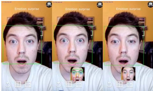
Fig. 5: Real-time detection of the emotion “Surprise” in three different intensities. The center images shows the regions used for landmark detection and the right image shows the obtained landmarks.
